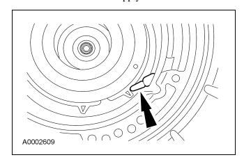
72. **CAUTION:** If the strut is installed incorrectly, transmission damage will occur.
